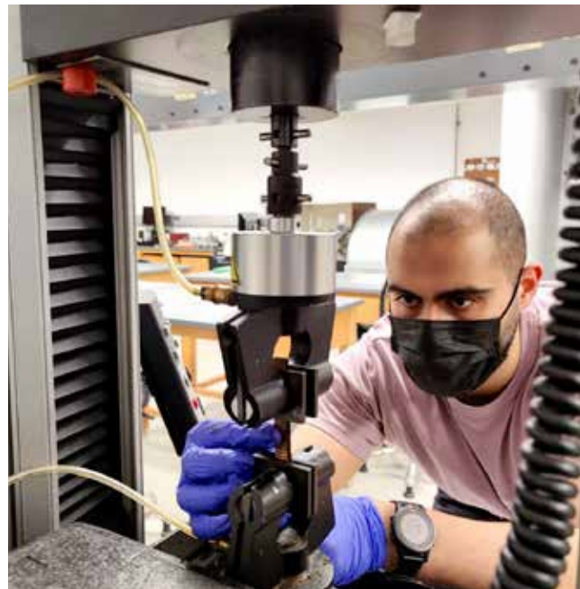
A graduate student tests the mechanical properties of the stubble-based composite panels. (Photo by Anil Netravali)
