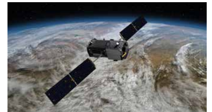
The Orbiting Carbon Observatory (OCO)-2 makes precise, regional measurements of carbon dioxide. (Image by NASA)
