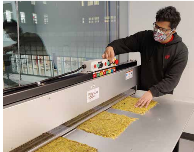
A member of Professor Anil Netravali's team operates the needle-punching machine that helps form mats out of rice straw and jute fabrics. (Photo by Abdullah Alkandary).
