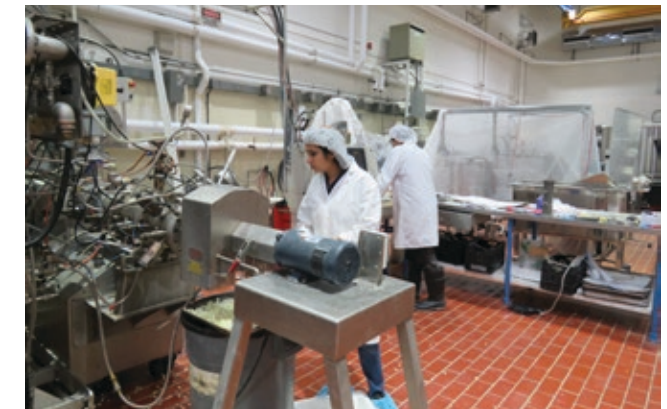
TCI scholar Bindvi Arora monitors the supercritical fluid extrusion system while producing a test batch of puffed snacks. (Photo by Dan Verderosa)
